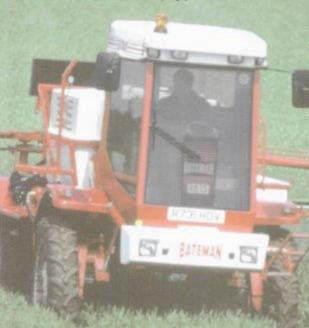
Application is controlled automatically via the LH AGRO 5000 computer linked to a pneumatic control system.
